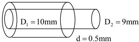
**MRR = cross section  $\times$  axial velocity**
