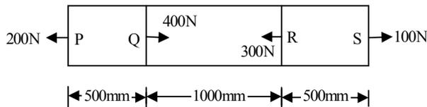
If  $E_{\text{steel}} = 200 \text{ GPa}$ , the total change in length of the rod due to loading is
