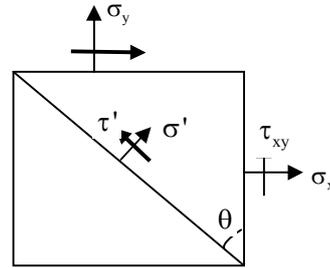
Max shear stress,  $\tau_{\max} = \sqrt{\left(\frac{\sigma_x - \sigma_y}{2}\right)^2 + \tau_{xy}^2}$
